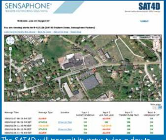
The SAT4D will transmit its status twice a day to the website. The status includes the present alarm condition of each input and the GPS location.
