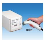
3 Continue holding down the button to decode and transmit bar code data.
