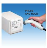
Press and hold the button to activate the laser line.
